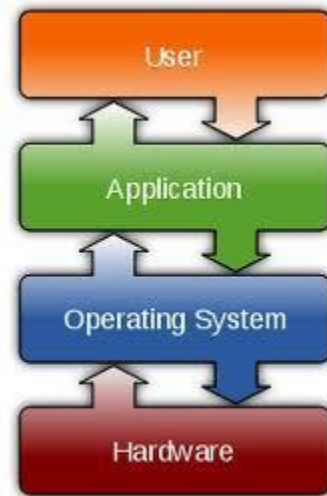
Figure 5: Diagram showing how operating system controls hardware, application programs and indirectly, users
